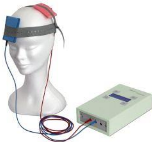
tCS device with an example of how the electrodes could be attached to your head
