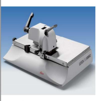
The Leica EMKMR2 glass knifemaker produces 45° glass knives from 6.4, 8 and 10 mm thick glass utilizing the balanced-break method. This method begins with a standard 400 mm long glass strip in any of the three thicknesses and continuously breaks the strip into equal halves. You then have a number of flat sided squares perfect for making 45° knives suitable for light and electron microscopy applications.
