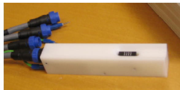
Figure 2.3: One of the piezoelectrical Braille stimulators. The stimulator contains a matrix of two columns by four rows of pins which are raised and lowered driven by a voltage.
