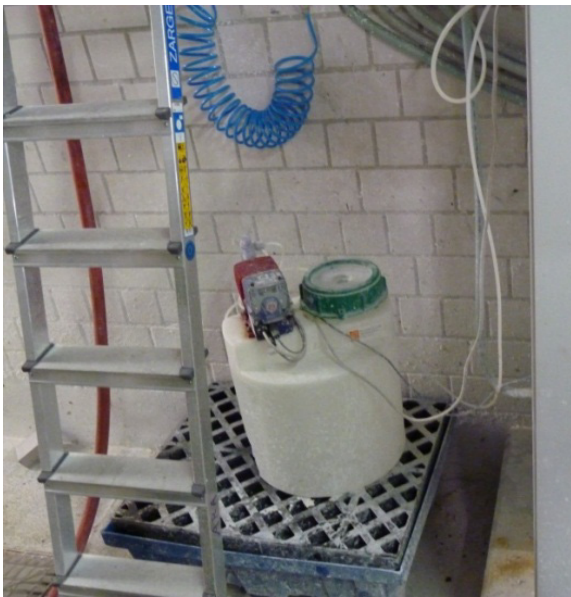
Fig. Acid Rinse option to clean tubes and sampling system
