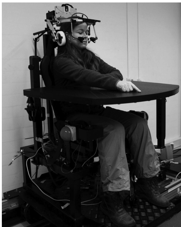
Fig. 1 Experimental setup. Subject seated in the sled, fixated with racing belts, headphones, and with the LED table in front performing reaching movements.
