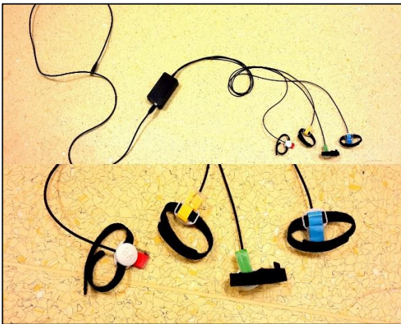
Fig 2. Color-coded accelerometers: target (yellow), opposite wrist (blue), ipsilateral leg (red), contralateral leg (green)
