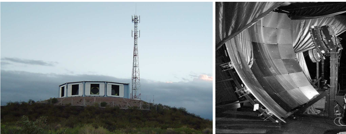
Figure 1.1: Left: The fluorescence station Los Leones. Each station contains 6 fluorescence telescopes. Right: A fluorescence telescope, the hollow mirror focuses the light on a photon multiplier camera.
