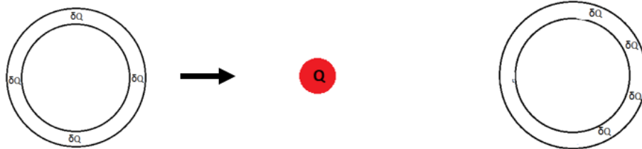
Figure 2.1: The surface charge distribution without (left) and with (right) and external body.
